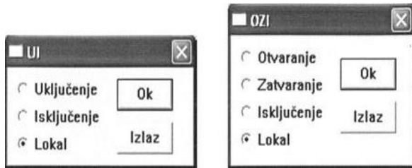
Fig. 3 Dialog menu with current selection and possible options for pump operation control valve actuator
