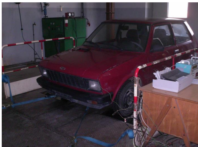
Fig. 1 Vehicle Yugo 1.3 CW on dynamometer roll SCHENK LNC-0052
