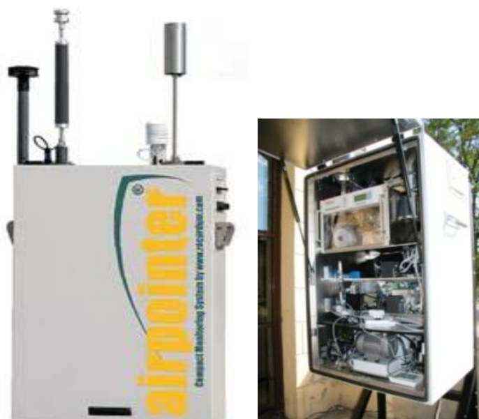
Fig. 1 Exterior and interior design of the measuring station “Airpointer”
