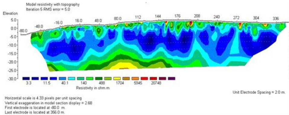
**Fig. 2** Interpreted 2-D Pseudosection along a profile running across the length of the area of study
