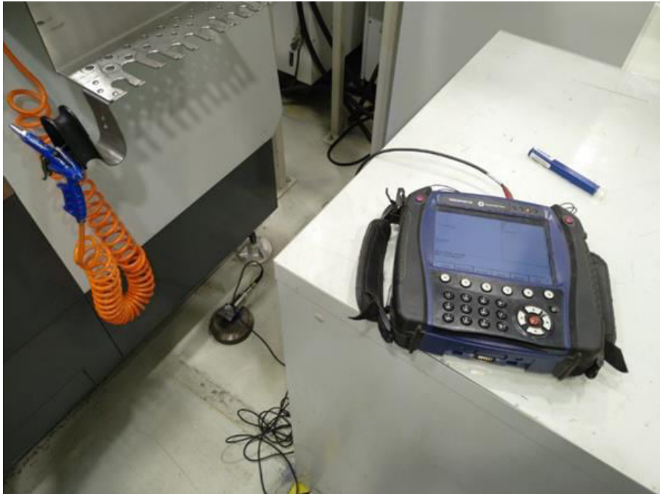
Fig. 4. Bruel&Kjaer Vibroport 80 with piezoelectric acceleration measuring cell AS-063
