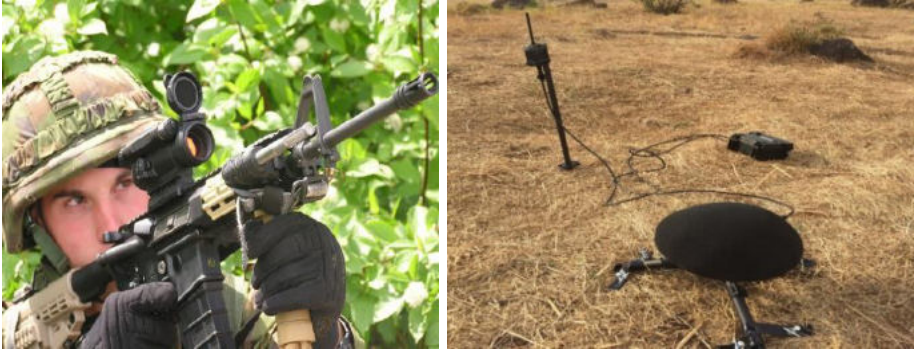
Fig. 2 A three-dimensional vector sensor mounted on the Colt C8 along with a miniature microphone [7] is shown on the left panel. On the right panel is the Ground-Based Gunshot Localization System – GBGLS, http://microflown-avisa.com/products/ground-based-gunshot-localisation/ , equipped with a similar sensor [8]
