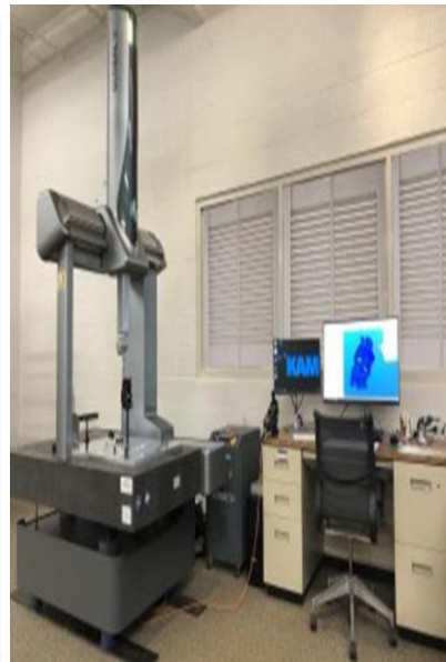
Fig. 1 a) Dimensions of the Hexagon Global S machine, b) appearance of the measuring machine in real space
