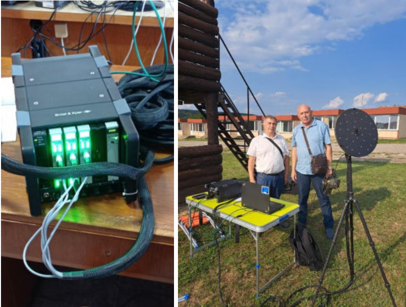
Fig. 4 Conducting measurements during a complex tactical exercise in the village of Belyakovets. The antenna array of a Bruel&Kaer acoustic camera is visible
