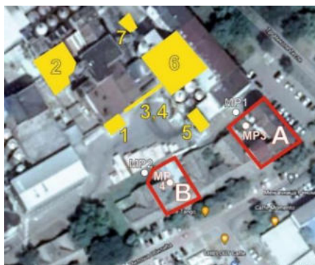
Fig. 2 Locations of noise sources in the brewery (positions 1 ÷ 7); Locations of areas in the environment affected by noise from the brewery (A and B); Locations of measurement points MP1 ÷ MP4 (Source: Google Earth)
